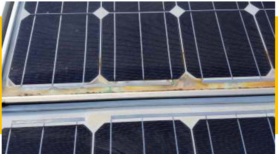
Four year old failed panel with water ingress
