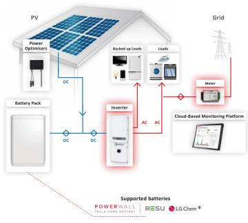
$^{*}$  LG Chem RESU battery will be supported with a different StorEdge Inverter, contact SolarEdge for details
